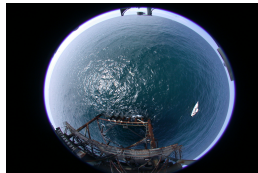
The "tower radiating effect". A fish-eye lens picture shows the structure in the field of view of the upwelling instruments. The signal from the tower is an undesired quantity. As shown in the photo to the left, the narrow field of view (FOV) IRT does not have the tower in its view. IRT specifications: 2.8° FOV, 9.6-11.5µm range.
