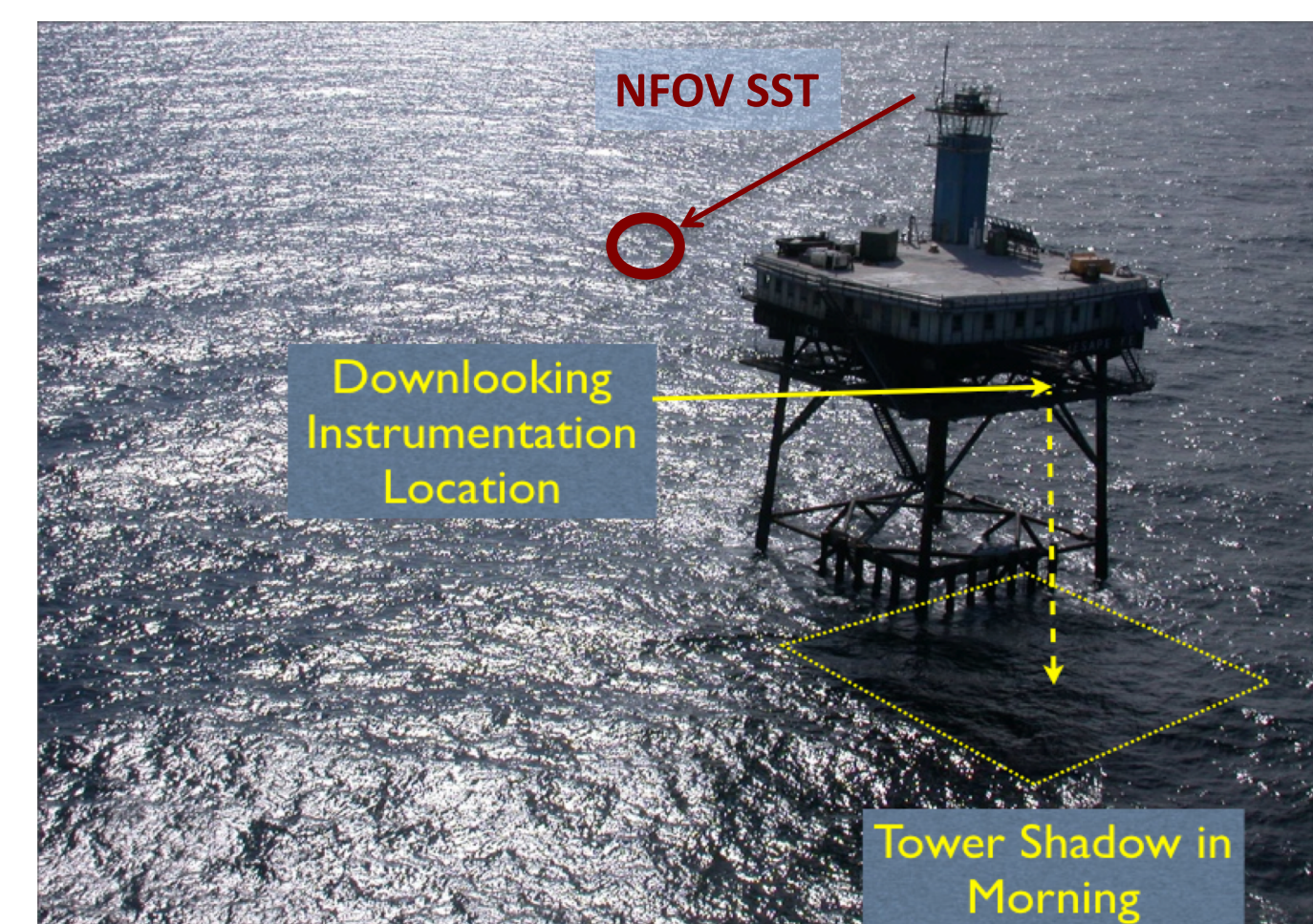
The "tower shading" effect. Notice the shaded area beneath the upwell instruments. This occurs primarily in the morning.
