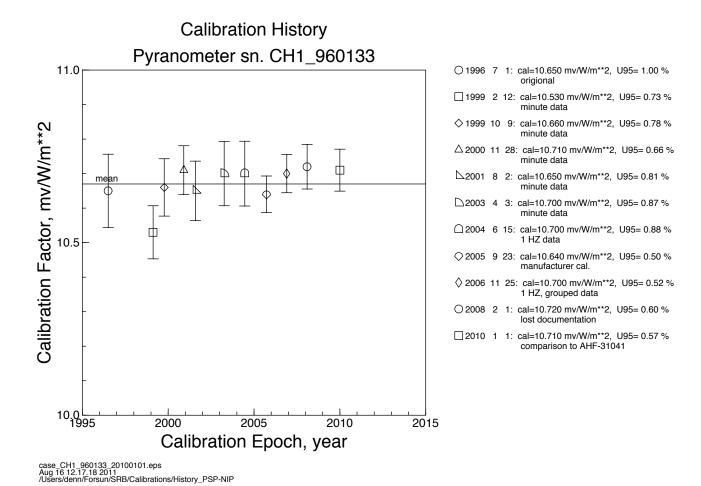
Figure 7. Calibration history for pyranometer CH1-960133 is presented. The solid horizontal line represents the mean value. The symbols and their error bars represent the mean and U95 of each calibration event. The column on the right presents numerical values for each calibration event and a brief description of the calibration method used.
