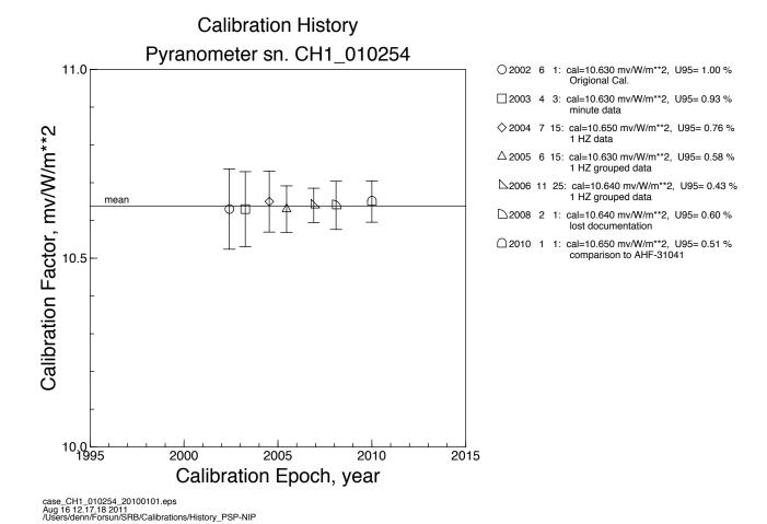
Figure 5. Calibration history for pyrheliometer CH1-010254 is presented. The solid horizontal line represents the mean value. The symbols and their error bars represent the mean and U95 of each calibration event. The column on the right presents numerical values for each calibration event and a brief description of the calibration method used.
