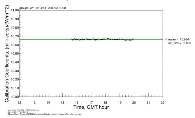
Figure 3. An example of selected calibration coefficients for CH1-010254, The data gaps occur while the cavity is self calibrating. The date between each gap will be combined into a single measurement. The date is on the top left of the plot.
