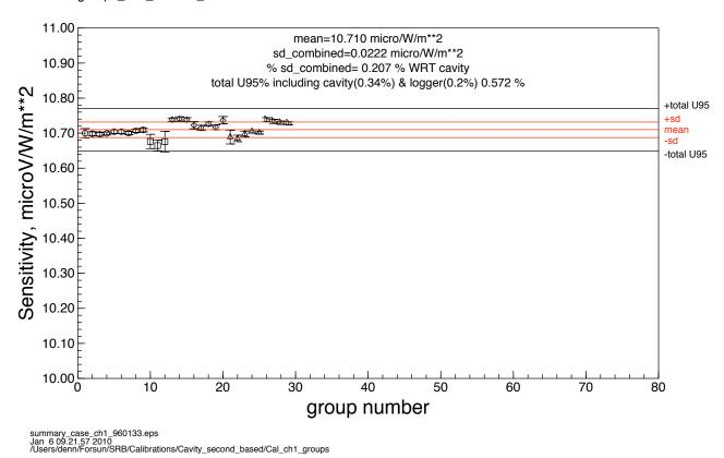
Figure 6. The data was grouped according to cavity run. A group must contain 66% of the maximum number of points possible. Data for CH1-960133 collected on five different dates are displayed. The dates are listed on the plot.
