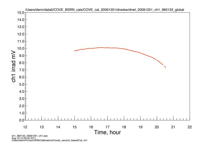
Figure 2. An example of millivolt measurements obtained by pyrheliometers CH1-960133. The date is in the line at the top of the plot and in the form yyyymmdd.
