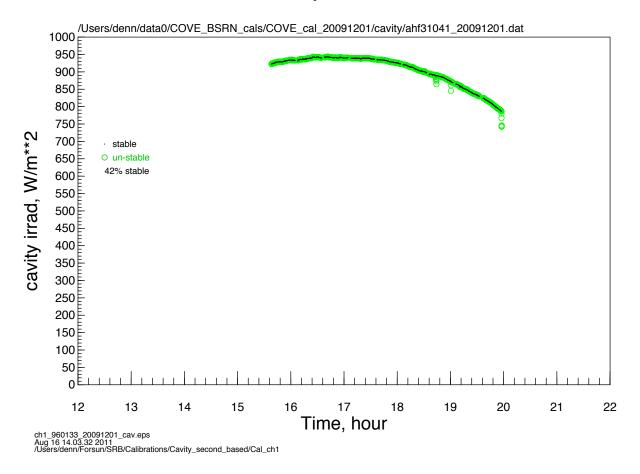
Figure 1. An Example of Irradiance measured by ACR AHF-31041. Note the gaps at approximately half hour intervals. The data gaps occur while the cavity system is doing its self calibration. Each set of data points between the gaps is considered to be a cavity run. The date is contained in the line at the top of the plot.
