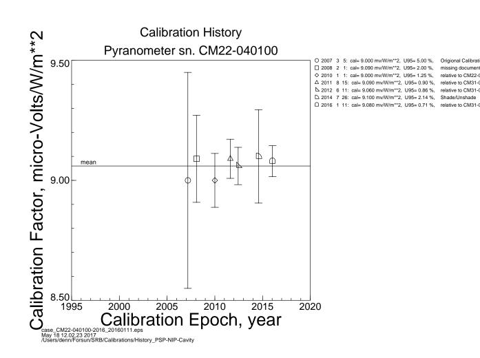
Calibration history for pyranometer CM22-040100. The solid horizontal line represents the mean value. The symbols and their error bars represent the mean and U95 of each calibration event. The column on the right presents numerical values for each calibration event and a brief description of the calibration method used.
