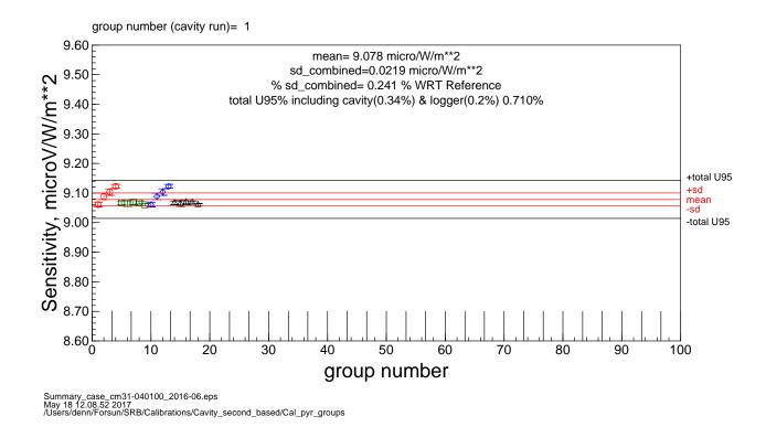
Calibration coefficients for several days. Each symbol represents a cavity run which is approximately 25 minutes. These data are combined to get a final calibration coefficient for the entire, multi-day, calibration session.
