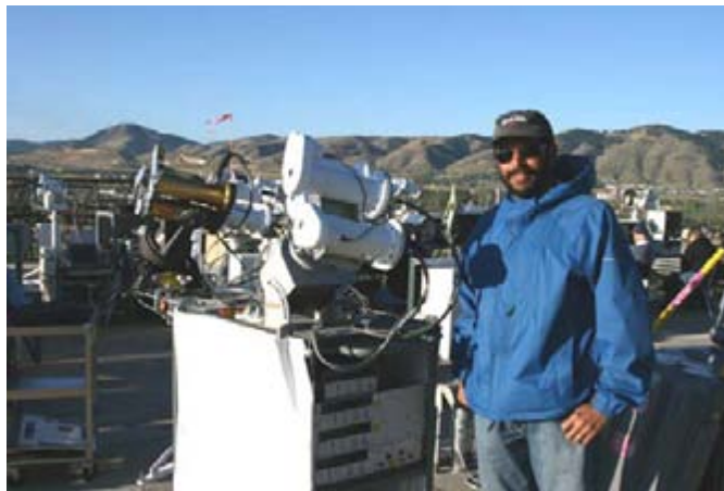
Figure ES-2. Ibrahim Reda operates NREL's absolute cavity radiometers on solar trackers. Four DOE/NREL reference standards were used to determine WRR-TFs for participating radiometers.
